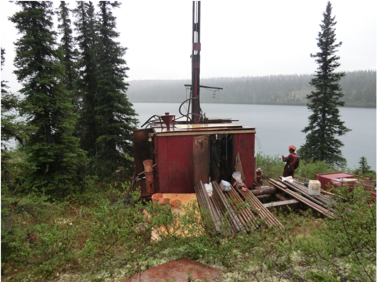
Figure 12 – RC Acker Drill Rig drilling hole Joy-12-111 – Cabo drilling
